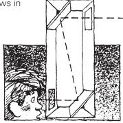
**Step 2:** Glue mirrors inside as shown in illustration. When you look through the bottom window you can see out the top.
